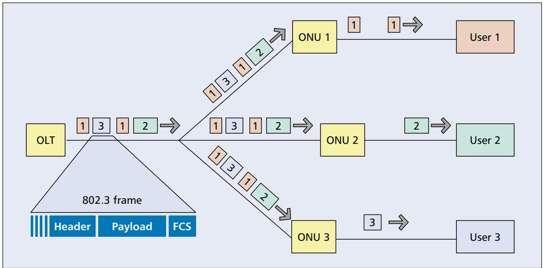
Figure 4. Downstream traffic in EPON.
