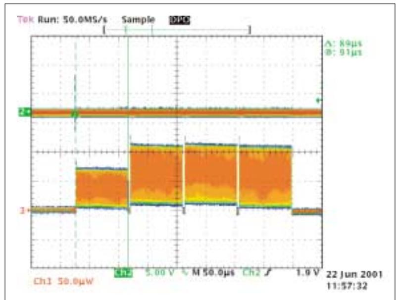
■ **Figure 6.** An illustration of the near-far problem: a snapshot of received power level from four ONUs.
